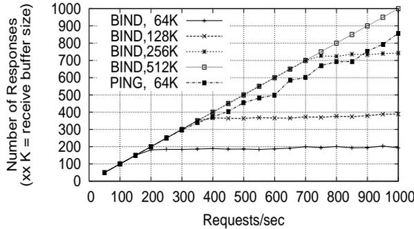
Figure 6: BIND 9.2.3 vs. PING with bursty traffic
