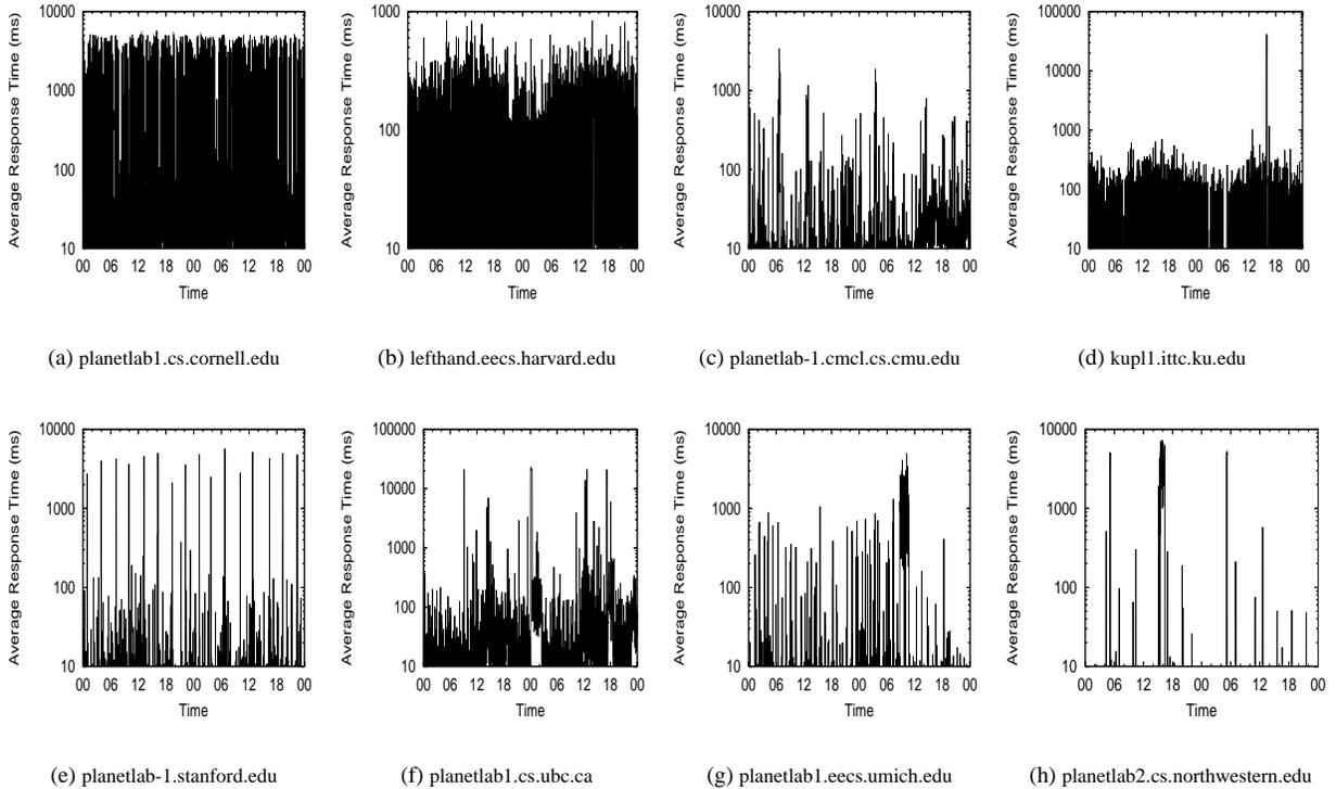
Figure 1: Average cached DNS lookup response times on various PlanetLab nodes over two days. Note that while most Y axes span 10-1000 milliseconds, some are as large as 100,000 milliseconds.
