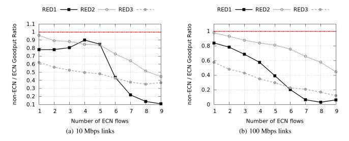
Figure 6: Unfairness between ECN and non-ECN flows for several flow-type mixes and RED parameter sets, given a constant number of 10 flows. In all parameter sets, the unfairness becomes larger when there are fewer remaining non-ECN legacy flows.
