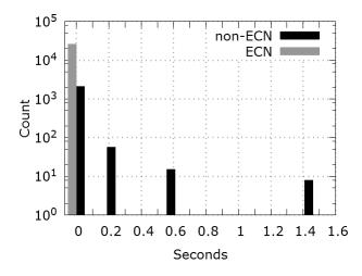
Figure 8: Histogram of time between consecutive acknowledgments sent by the receiver, divided into 100 ms bins, given a single non-ECN flow competing with 9 ECN flows on a 100 Mbps link. A representative ECN flow is plotted along with the non-ECN flow.
