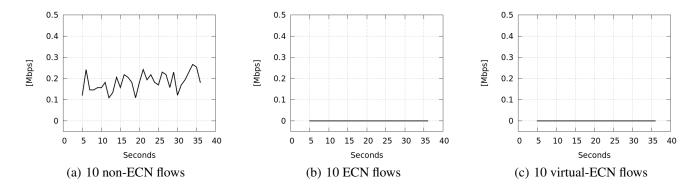
Figure 10: Total retransmission throughput for (a) 10 concurrent non-ECN flows sharing a 10 Mbps link, compared to the same experiment with (b) 10 concurrent ECN flows, and (c) 10 concurrent virtual-ECN flows.
