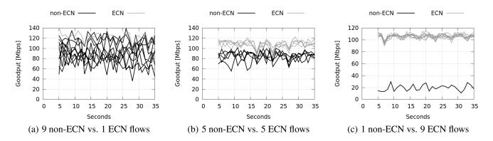
Figure 5: Repeated unfairness test between ECN and non-ECN flows with a 1 Gbps bottleneck link.
