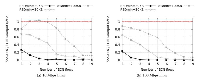
Figure 7: Average goodput ratio with varying values of RED<sub>min</sub>, given 10 senders. Increased numbers of ECN flows lead to starvation of non-ECN flows.
