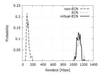
Figure 1: 10 flows share the same bottleneck link: an ECN-unaware flow (non-ECN), 8 ECN-enabled flows (ECN), and a non-ECN flow augmented by vCC translation (virtual-ECN). The figure plots the probability density function, over many runs, of the average goodput of each flow. The non-ECN flow is starved, reaching only 10% of the ECN goodput on average. After translation to virtual-ECN, the average goodput is near identical to that of ECN.
