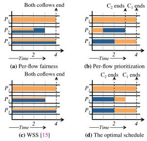
**Figure 2:** Allocation of *ingress* port capacities (vertical axis) using different mechanisms for the coflows in Figure 1. Each port can transfer one unit of data in one time unit. The average FCT and CCT for (a) per-flow fairness are 3.4 and 4 time units; (b) per-flow prioritization are 2.8 and 3.5 time units; (c) Weighted Shuffle Scheduling (WSS) are 3.6 and 4 time units; and (d) the optimal schedule are 3 and 3 time units.
