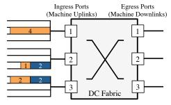
**Figure 1:** Coflow scheduling over a  $3 \times 3$  datacenter fabric with three ingress/egress ports. Flows in ingress ports are organized by destinations and color-coded by coflows –  $C_1$  in orange/light and  $C_2$  in blue/dark.
