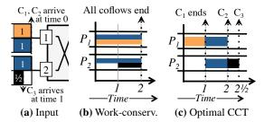
Figure 15: Allocation of ingress port capacities (vertical axis) for the coflows in (a) on a 2 × 2 datacenter fabric for (b) a work-conserving and (c) a CCT-optimized schedule. While the former is work-conserving and achieves higher utilization, the latter has a lower average CCT.
