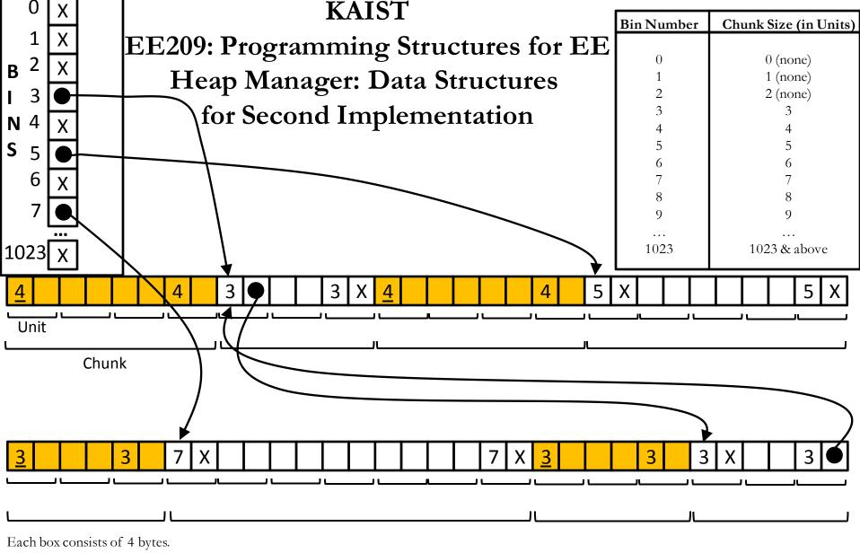
Each Chunk's header Unit contains a status (INUSE or FREE), a length, and, if the Chunk is free, a pointer to the next Chunk in its Bin. Each Chunk's footer Unit contains a length and, if the Chunk is free, a pointer to the previous Chunk in its Bin.
