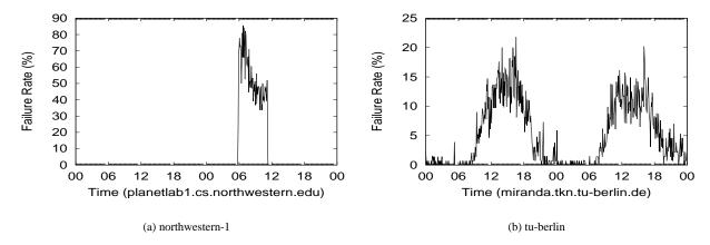
Figure 4: Failures seemingly caused by nameserver overload – in both cases, the failure rate is always less than 100%, indicating that the server is operational, but performing poorly.
