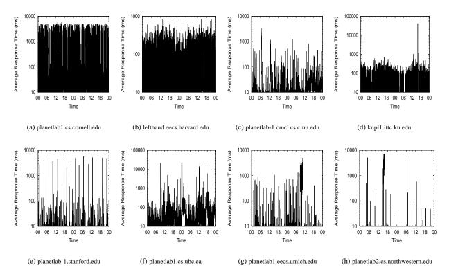
Figure 1: Average cached DNS lookup response times on various PlanetLab nodes over two days. Note that while most Y axes span 10-1000 milliseconds, some are as large as 100,000 milliseconds.
