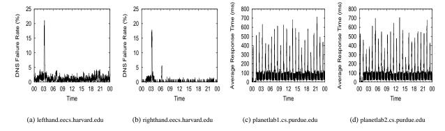
Figure 3: All nodes at a site see similar local DNS behavior, despite different workloads at the nodes. Shown above are one day's failure rates at Harvard, and one day's response times at Purdue.
