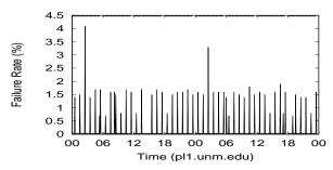
Figure 7: This site shows failures induced by periodic activity. In addition to the hourly failure spike, a larger failure spike is seen once per day.
